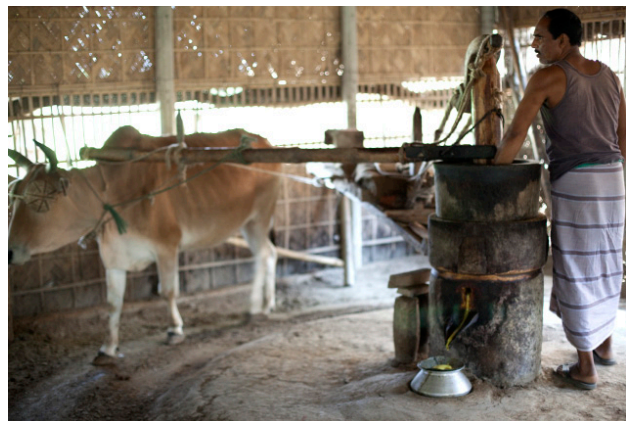
Full view of traditional pressing machine. Notice the mustard seed oil dripping into the metal vessel, just like main photo above.
